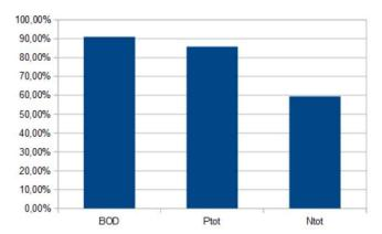
The purification efficiency of the **grey water** purification was 91 % for BOD, 86 % for Ptot and 59 % for Ntot.
