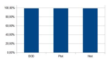
According to **official calculating method (which includes also the load of toiletswaters)** used in legislation in Finland and in Sweden the purification was 99 % for BOD, 99 % of Ptot and 99 % of Ntot.
